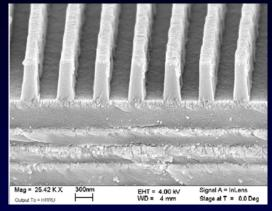
$\begin{array}{l} \mbox{multi-layer dielectric diffraction} \\ \mbox{grating, NIF lasers (LLNL)} \\ \mbox{$2 \times 10^6$ periods!} & (\mbox{Barty '04}) \end{array}$
